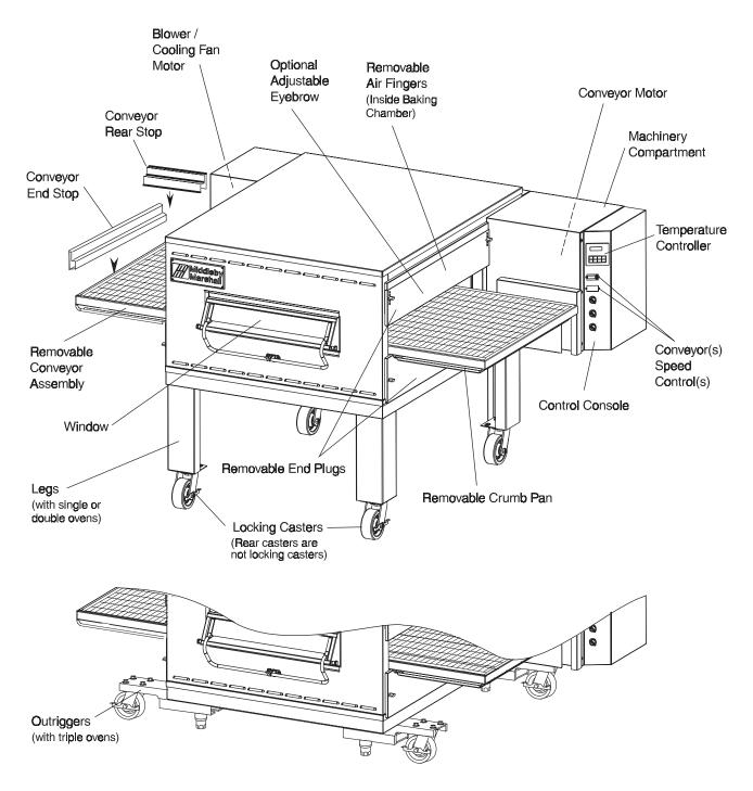
Figure 1-6. PS540-Series Oven Components Locations
